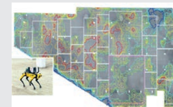
Evaluation of the flatness of concrete slab utilizing a robot
